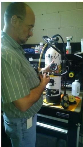
Regulators contain numerous O-rings, Diaphragms; high and low pressure seats and hoses. These are critical to the regulator’s ability to function safely. Over time, these can dry out, oxidize, shrink and crack. This occurs regardless of whether the regulator is used or not. A regulator pressure seat “sits” on the orifice ALL the time until you take a breath. It is digging into the seat just sitting in your garage or closet.
